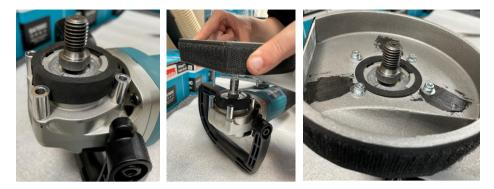
Step 04:Insert backing flange, keeping extra milled edge outward (to take cup wheel). Fit washer and nut.(Note: When fitting a cup wheel, the washer must go on the outside with the nut!)
